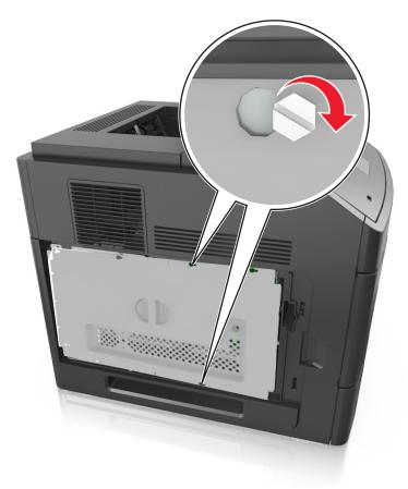
**7** Reattach the controller board access cover.
